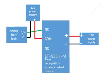
• Wiring to access controllers (take ER-SR22 as an example)
